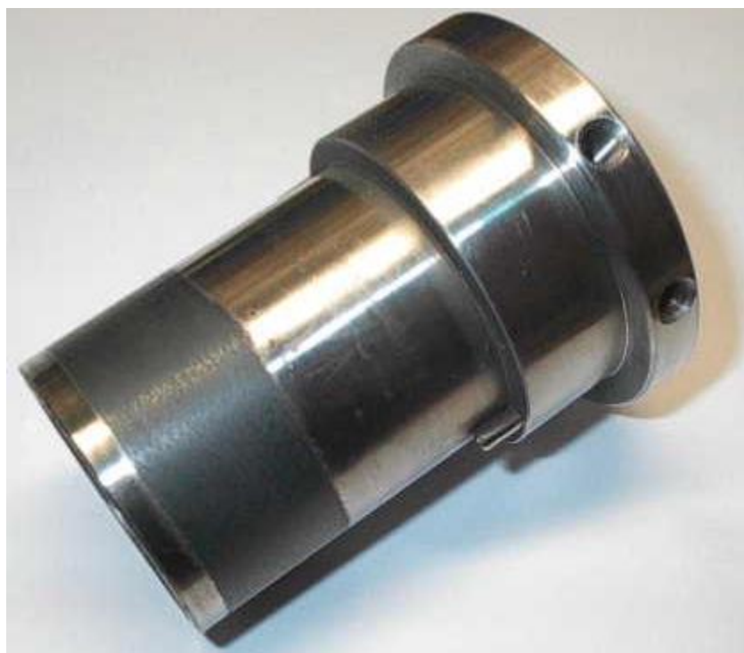
Figure 5. Sleeve coated with B 4 C, ground, then polished.
