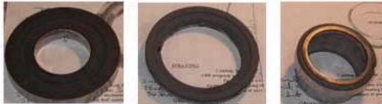
Figure 1a. Pump mechanical seals coated with B4C, ground, then lapped
