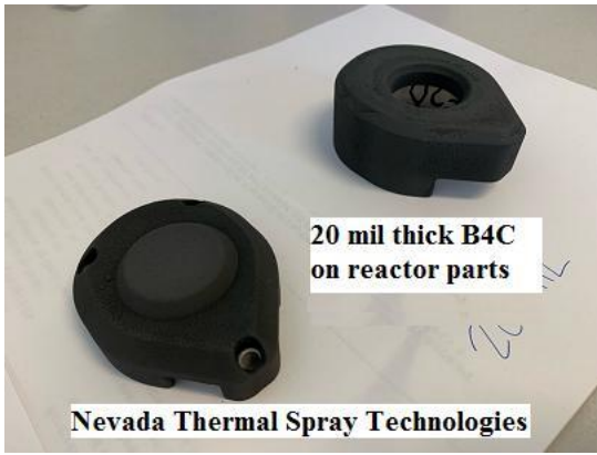
Figure 6. Reactor parts coated with B4C.
