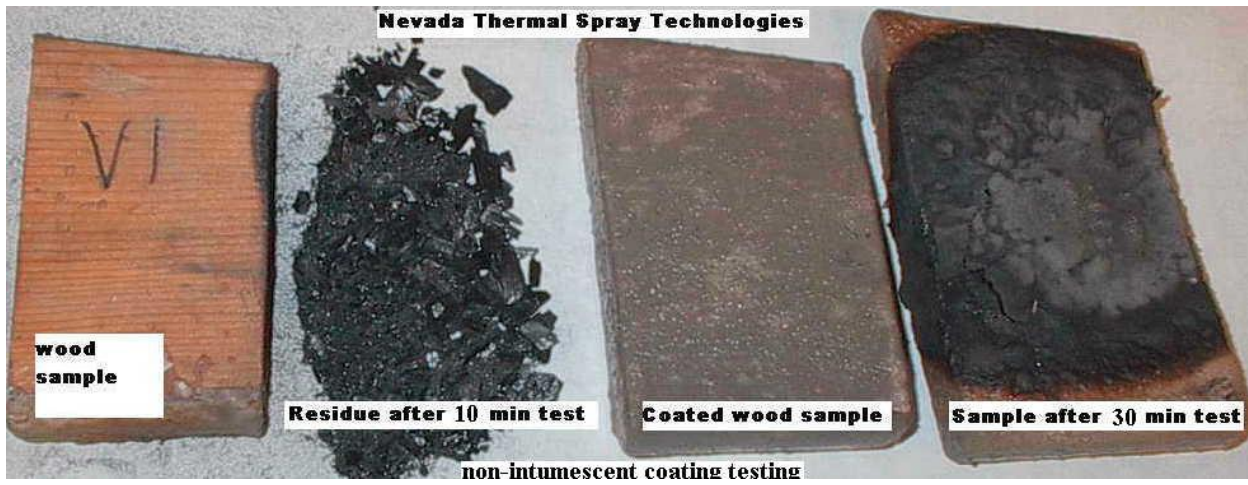
Figure 4. NTST Fire Protection Non-Intumescent Coating 30 Minute Test on Wood.
